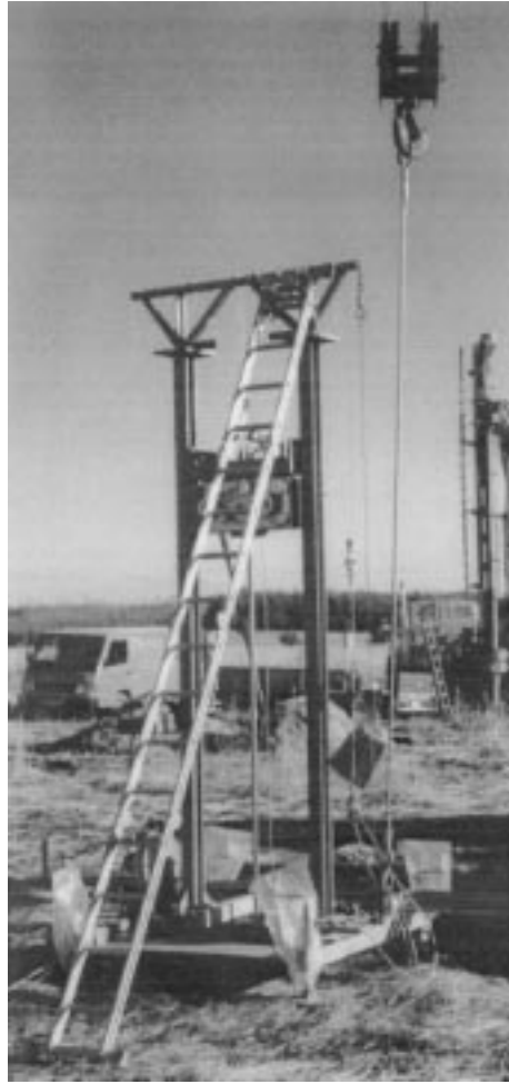
Figure 4. Set-up for vibratory sounding.
